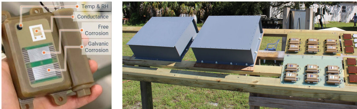
Figure 2. Environment and corrosivity monitoring device (left) and test rack at the Battelle IC site with monitoring devices and SAS boxes (right).
